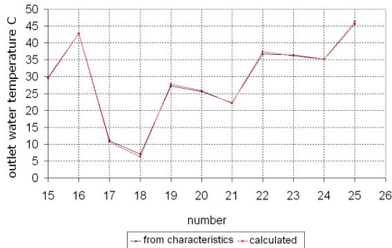
Figure 5: Change in water temperature at the outlet of the steam condenser, from characteristics and calculated for the next 11 values
