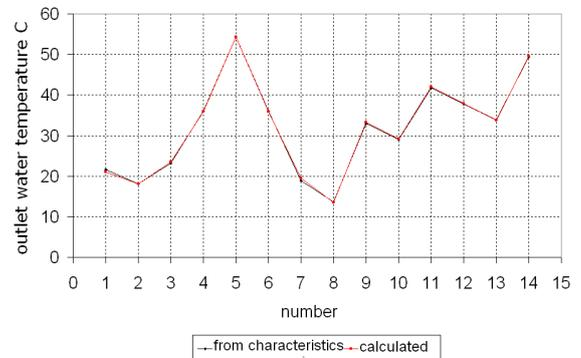
Figure 4: Change in water temperature at the outlet of the steam condenser, from characteristics and calculated
