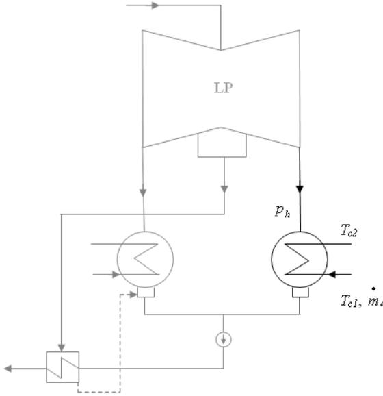
Figure 1: Location of the analyzed steam condenser in a 200 MW power plant with accepted symbols
