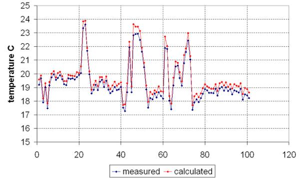
Figure 11: Change in water temperature at the outlet of the steam condenser, measured and calculated for 100 values at the end of the year
