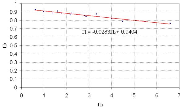
Figure 2: A comparison between two dimensionless quantities (data from the characteristics of the steam condenser)
