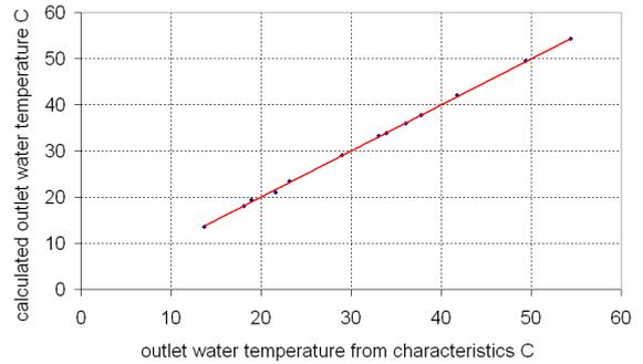
Figure 3: A comparison between water temperature at the outlet of the steam condenser, from the characteristics and calculated (21)
