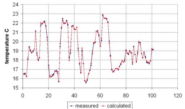
Figure 8: Change in water temperature at the outlet of the steam condenser, measured and calculated for 100 values at the beginning of the year
