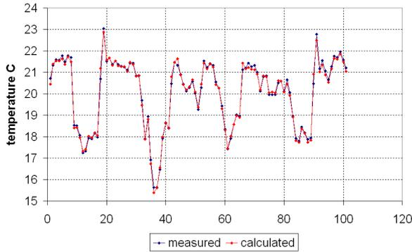
Figure 9: Change in water temperature at the outlet of the steam condenser, measured and calculated for the next 100 values
