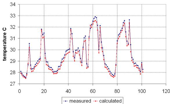
Figure 10: Change in water temperature at the outlet of the steam condenser, measured and calculated for 100 values in the middle of the year
